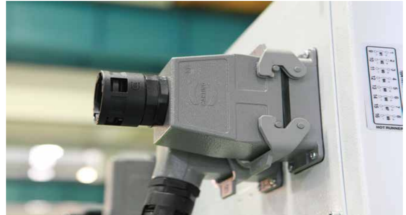
▶ EUROMAP 67 based program and plug for robot
