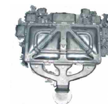
高速压射容易产生飞边 High speed injection causing flush
