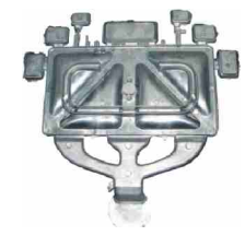
末端刹车功能有效减少飞边 Injection end brake function reducing the flush effectively
