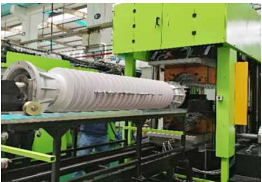
制品名称：220kV管套 成型腔数：一出二 Part Name: 220 kV Hollow Core Insulator Number of Cavities: 1
