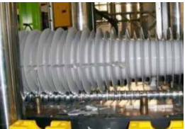
制品名称：110kV锥形管套 成型腔数：一出二 Part Name: 110kV Cone Type Hollow Core Insulator Number of Cavities: 1
