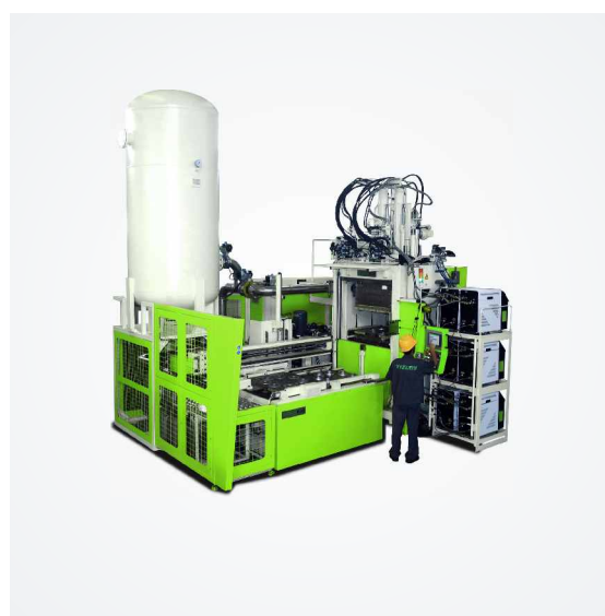
YL-VV450F (双物料注射机) (Dual-material injection machine)
