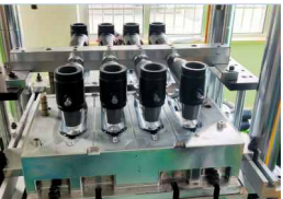
制品名称：10kV T型接头 成型腔数：一出八 Part Name: 10kV T Joint Number of Cavities: 8
