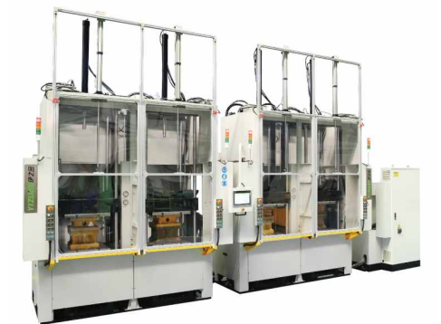
YL-V50 膜式空气弹簧硫化成型机 Rolling lobe air spring molding machine
