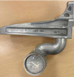
Weight: 14 kg (Replacing gravity casting with a T6 to simplify machining)
