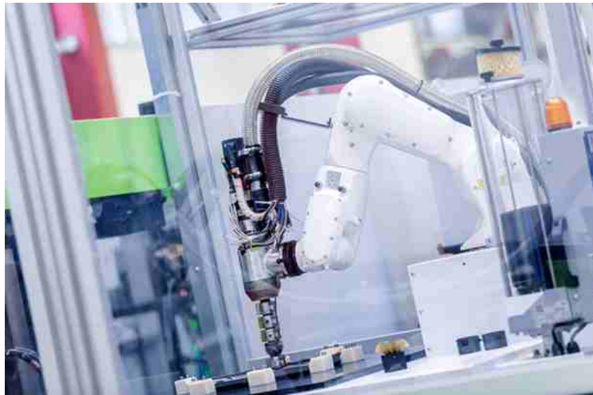
Fig. 3: Small SpaceA Printer inside of an automated manufacturing cell to functionalise a moulded part – your cost-efficient way in the business of Multi-Material Part Production
