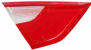
Part: Two-color Taillight Cover Model: UN750C-BTP Number of cavities: 2+2 Material: PMMA + PMMA Part size(L×W×H): 252 x 158 x229mm Part weight: 82g Cycle time: 50s
