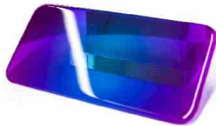
Part: Mobile Phone Back Frame Model: FF160 Number of cavities: 1 Material: PC Part size(L x W): 158x78 mm Part weight: 17.7g Wall thickness: 0.7mm Cycle time: 25s
