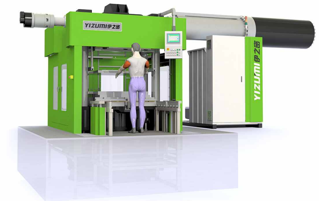
YL2-AB1200L ( Injection volume 40000cm 3 , injection pressure 1900bar )
