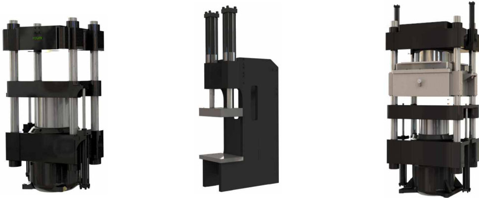
D2 Structure: 4-column 2-step upward closing; Features: Simple, full stroke clamping available. D4 Structure: C-frame 2-step downward closing; Features: Column free structure, 3-side operation accessible, double sliding plate or rotary table available to achieve double lower mold exchange; Downward closing structure, inserts will not move. D6 Structure: 4-column 2-step upward closing with vacuum chamber; Features: Avoid air trapping, ideal for products with complex structure, no need for venting during injection, less flash.
