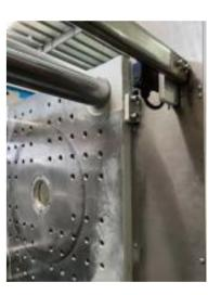
The lower part of the product dropping area is covered with stainless steel plates, which is clean and wear-resistant.
